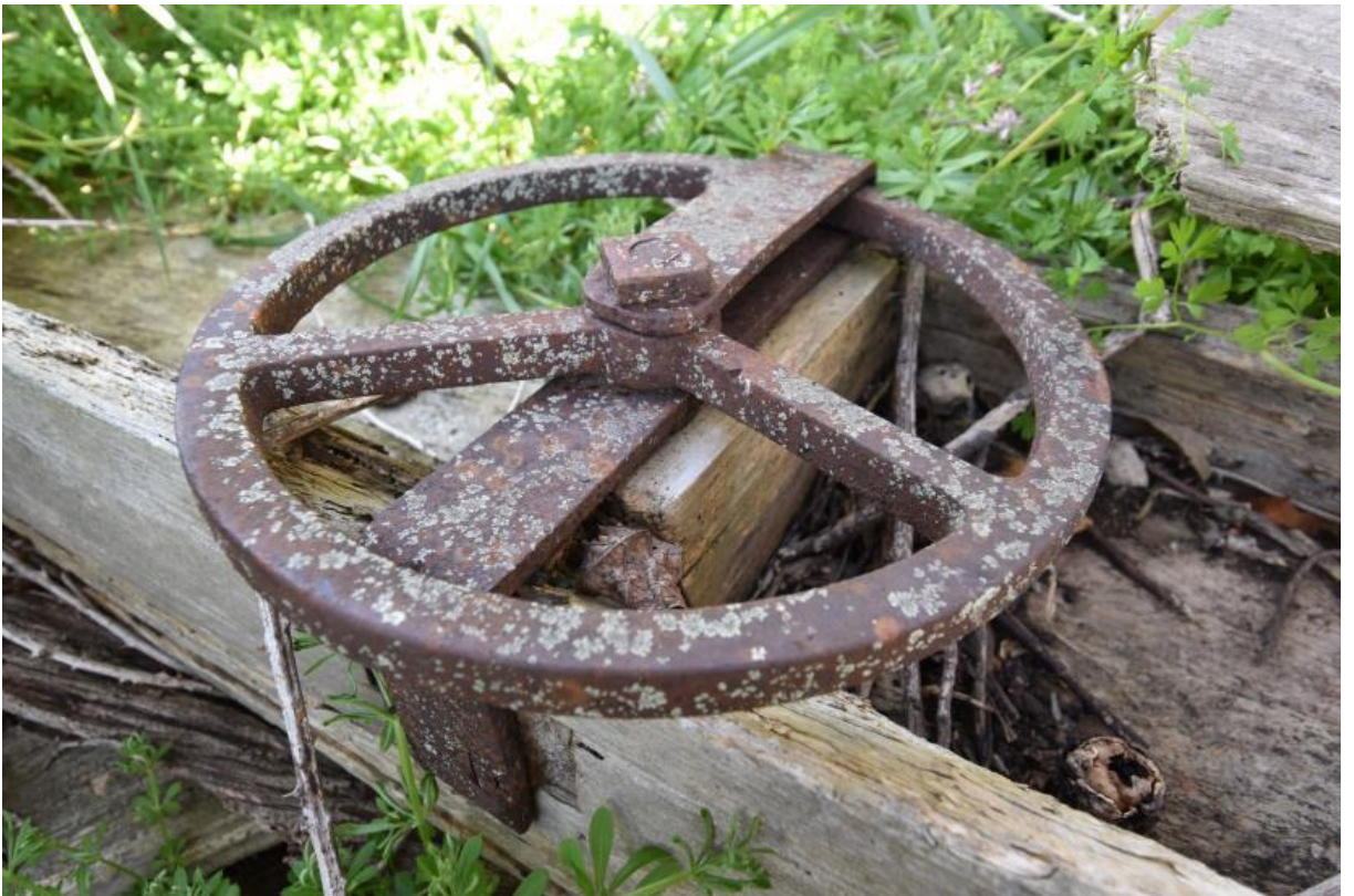
Figure 8. Example of an iron wheel, part of the mechanism which allowed the canvas dome of the equatorial room to revolve when in situ. It is now on the ground in the transit annex. Kerry Pollock, Heritage New Zealand Pouhere Taonga, 12 September 2019.
